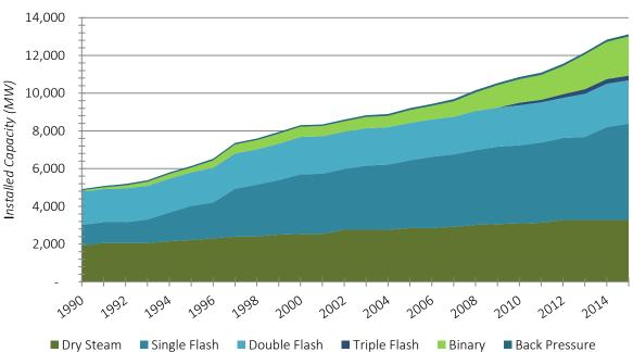
Figure 9: Operating Capacity by Technology Type
