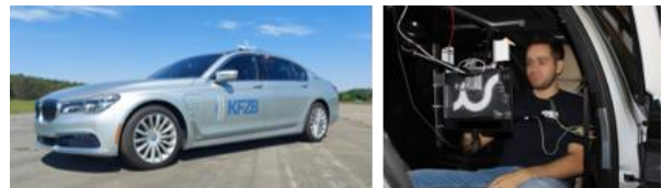
Fig. 1 Experimental vehicle (left) and passenger cabin with tablet, camera and devices to measure vital-parameters (right)
