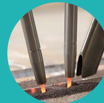
Tandem (LSO) process in operation and inside typical offshore monopile weld joint
