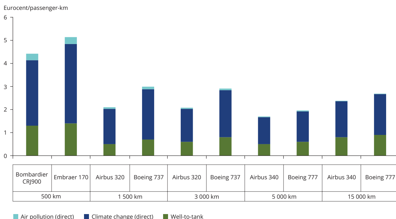
Figure 3.11 Marginal costs of air pollution, climate change and well-to-tank emissions of passenger air transport for selected cases
