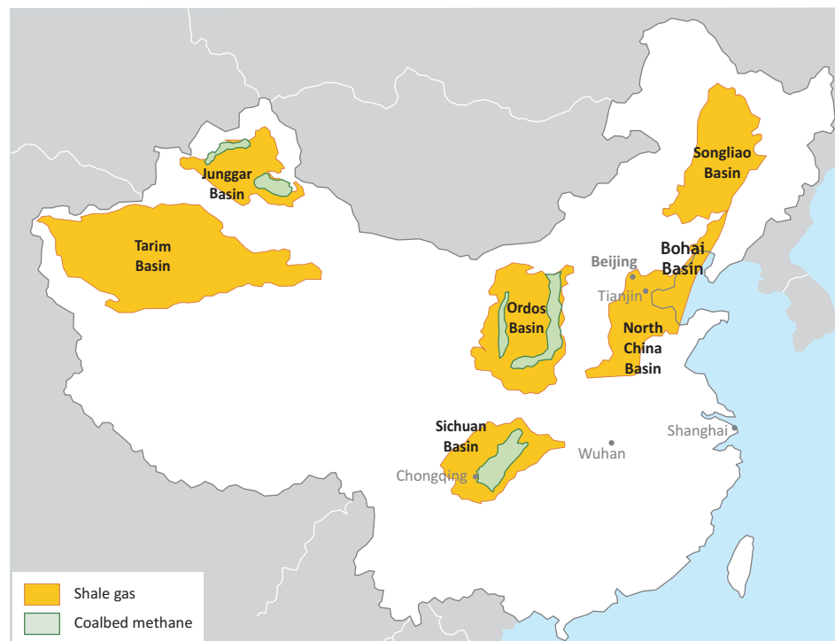
Figure 3.5 ▶ Major unconventional natural gas resources in China
