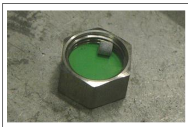
Figure 2- 50 : Pastille Futurix non irradiée, Pu_{0,5}Am_{0,5}O_{2-\delta}-MgO
