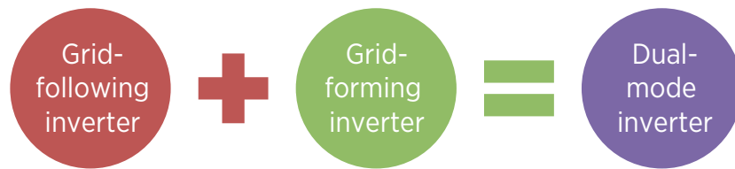
Figure 5: Relationship between grid-following, grid-forming and dual-mode inverters
