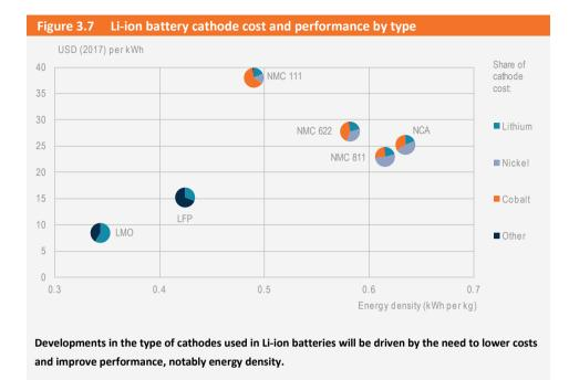
Notes: kWh = kilowatt hours. Energy density is for the cathode only. Cathode costs account for a varying share of battery pack costs. For NCA and NMC cathodes, the share is 50% to 60%. Numbers represent the ratios of the metals in the cathodes if there are different variants.
