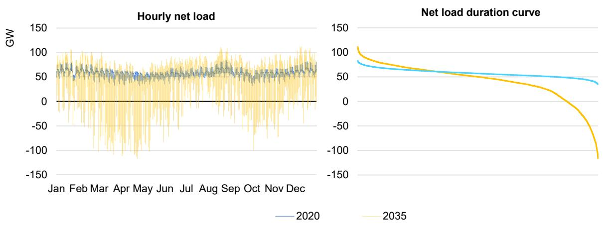
Note: Net load = total load minus wind and solar power generation.
