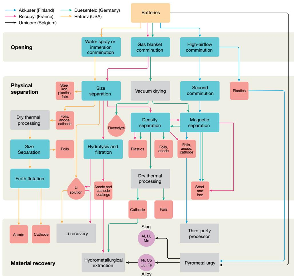
**Fig. 5 | Flow chart representing potential routes for the circular economy of LIBs, detailing second-use applications, re-use, physical recovery, chemical recovery and biorecovery.** A range of commercial entities have
