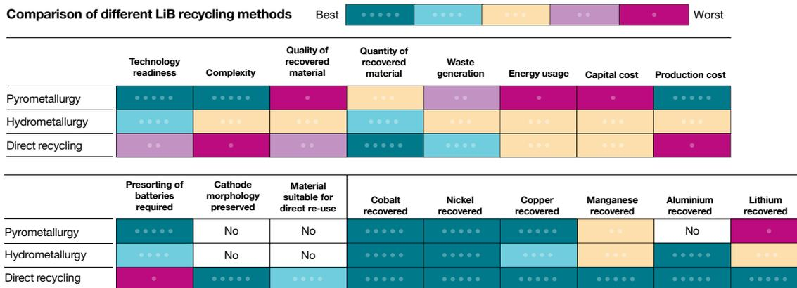
**Fig. 6 | Comparison of different LiB recycling methods.**
