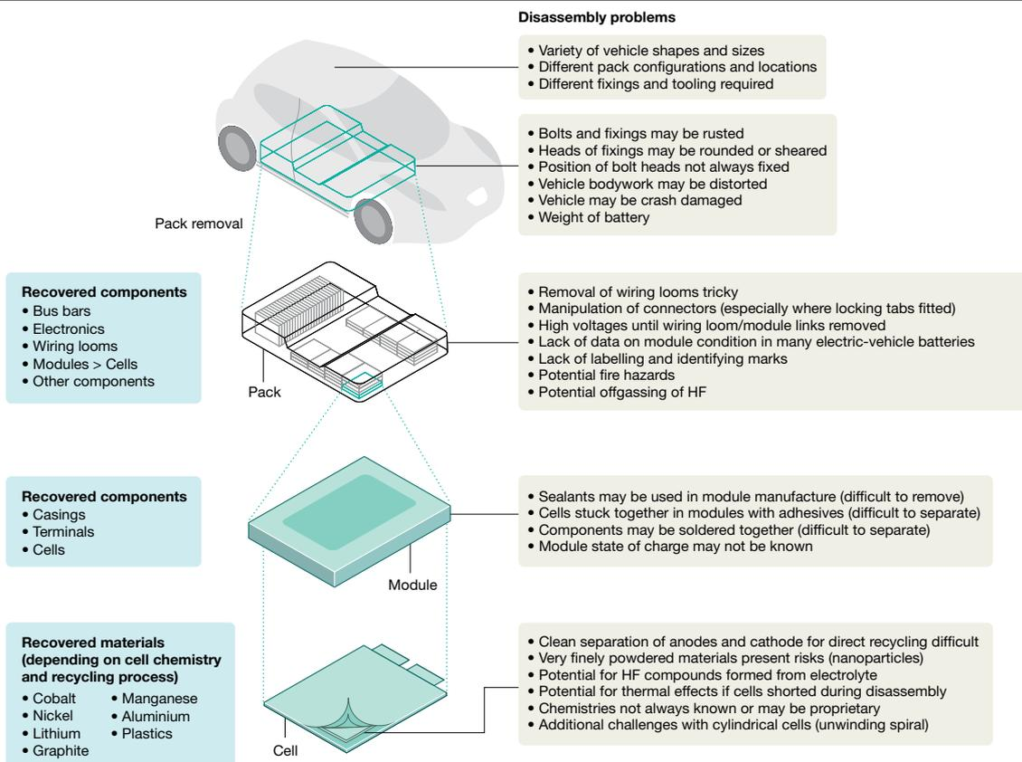
**Fig. 4 | Diagram showing challenges of disassembly at different levels of scale.** Electric-vehicle battery packs are complex in design, containing wiring looms, bus bars, electronics, modules, cells and other components. There are
