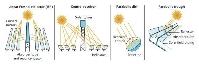
KEY POINT: Most current CSP plants are based on trough technology, but tower technology is increasing and linear Fresnel installations emerging.
